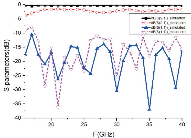
Figure 4 The simulated and measured results of the coaxial-to-ridge waveguide adapter.
