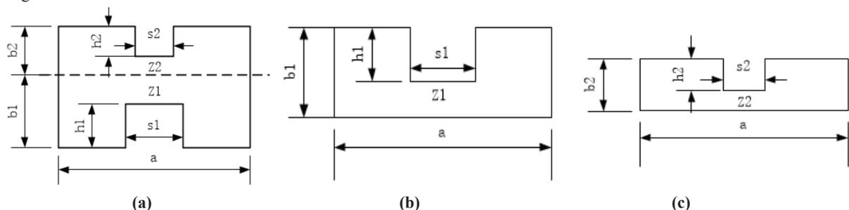
Figure 1 The asymmetrical double ridge waveguide. (a) Top view, (b) left-side view, and (c) right-side view.
