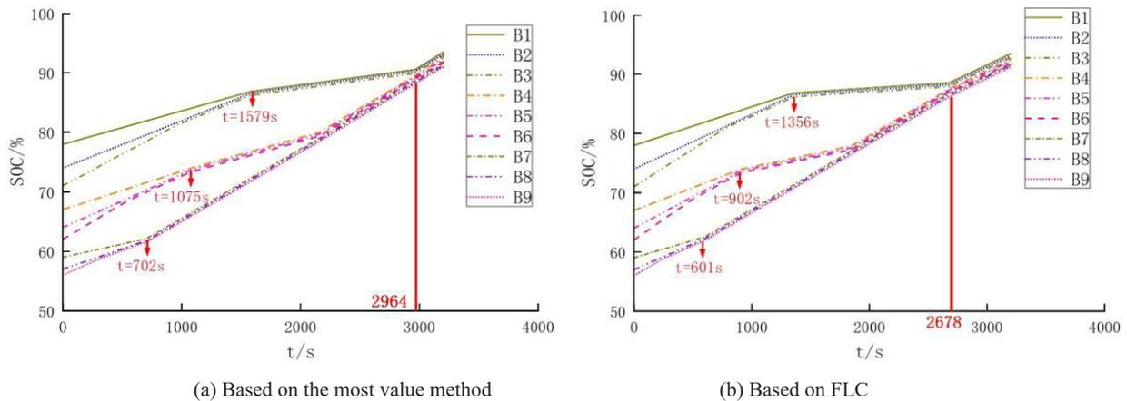
Fig. 7 Variation of battery SOC under charging equalization
