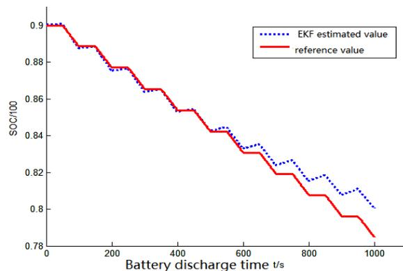
Fig. 3 SOC estimation based on EKF algorithm
