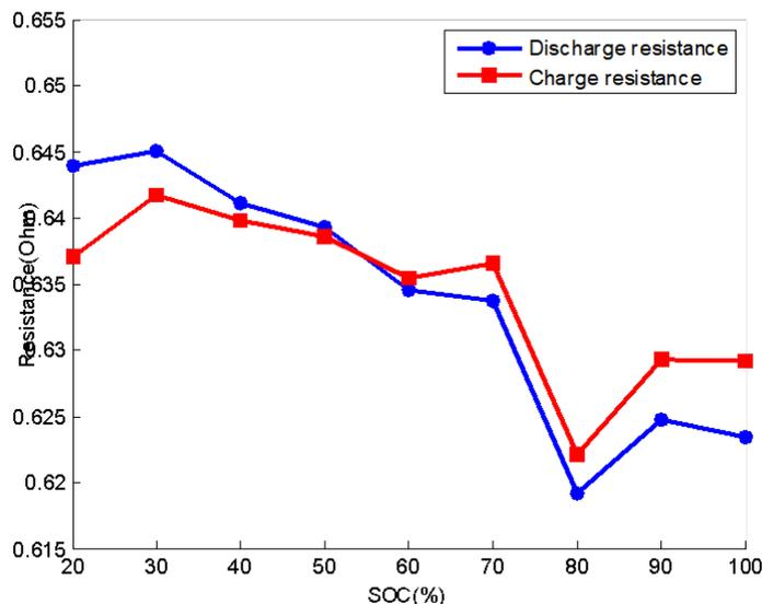
Fig. 1 Charge/discharge internal resistance of battery corresponding to different SOC levels
