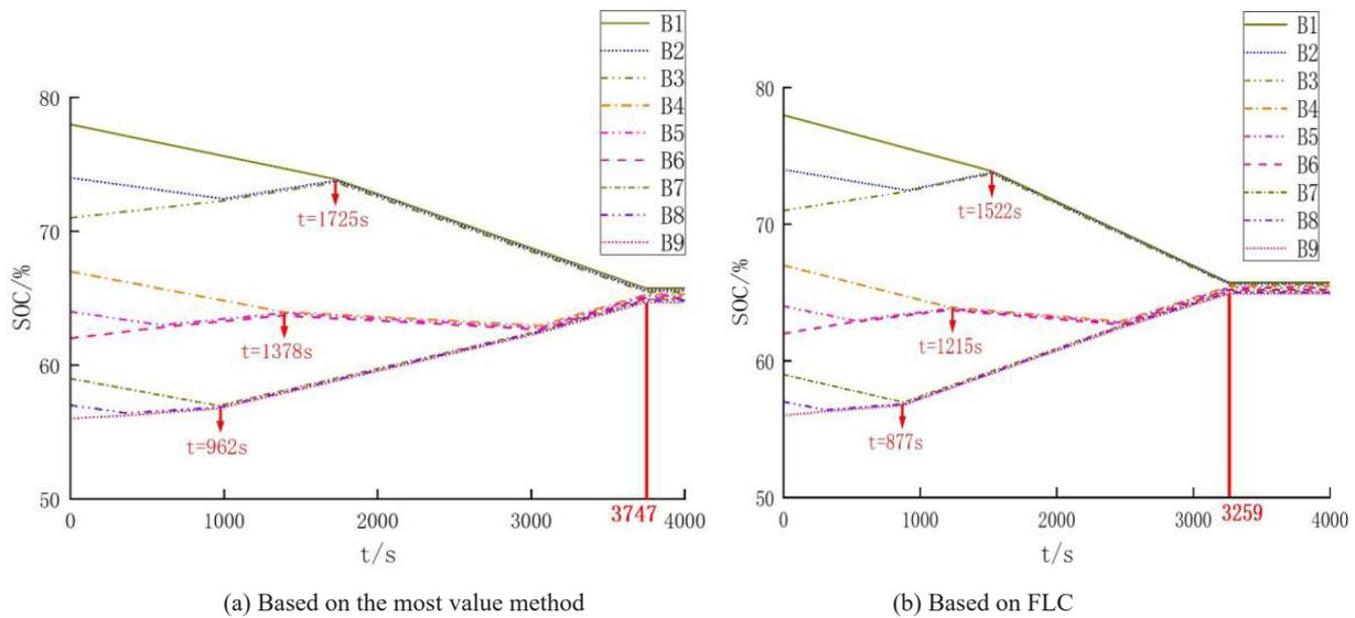
Fig. 6 Variation of cell SOC under static equalization
