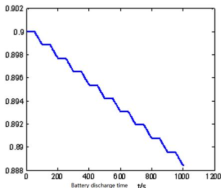
Fig. 2 SOC estimation based on EKF
