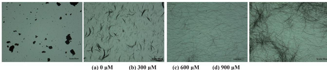
Fig. 2 Surface optical microscope images of Ag NWs films prepared under different concentrations of  $\text{FeCl}_3 \cdot 6\text{H}_2\text{O}$  solutions.
