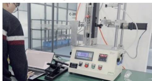
Figure 3. Lock handle testing equipment
