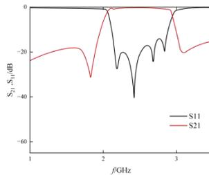
Fig.3 Simulation result of wideband filter
