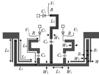
Fig.5 Geometry of the bandwidth tunable optical filter ( $L_1=16.25$  mm,  $L_2=12$  mm,  $L_3=0.5$  mm,  $L_4=4.85$  mm,  $L_5=11.25$  mm,  $L_6=8$  mm,  $W_1=0.5$  mm,  $W_2=0.3$  mm,  $W_3=W_4=W_5=0.5$  mm,  $W_6=0.3$  mm,  $g_1=g_2=0.15$  mm)
