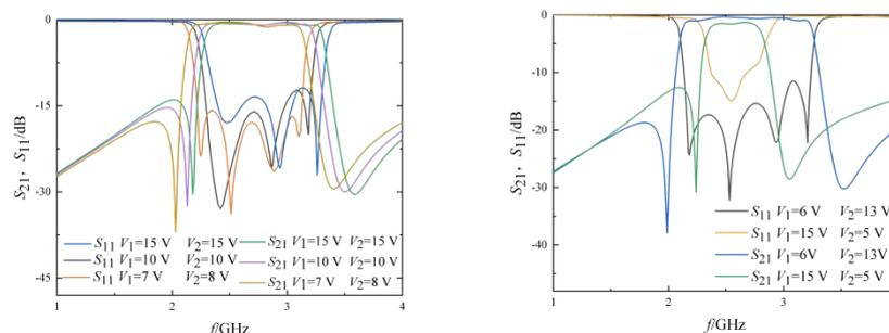
(a) Effect of V1 and V2 on the passband bandwidth (b) Effect of V1 and V2 on the center frequency
