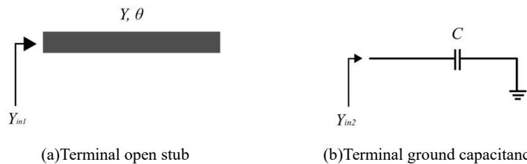
Fig.4 Open stub and terminal ground capacitance
