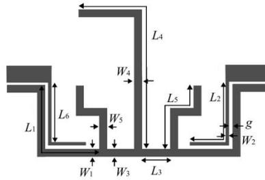
Fig.2 Geometry of the Wideband filter. ( $L_1=15.61$  mm,  $L_2=13.8$  mm,  $L_3=1.3$  mm,  $L_4=27.5$  mm,  $L_5=15$  mm,  $W_1=0.5$  mm,  $W_2=0.3$  mm,  $W_3=W_4=W_5=0.5$  mm,  $g=0.15$  mm)
