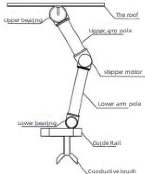
**Fig. 4 structure diagram of double link manipulator**
