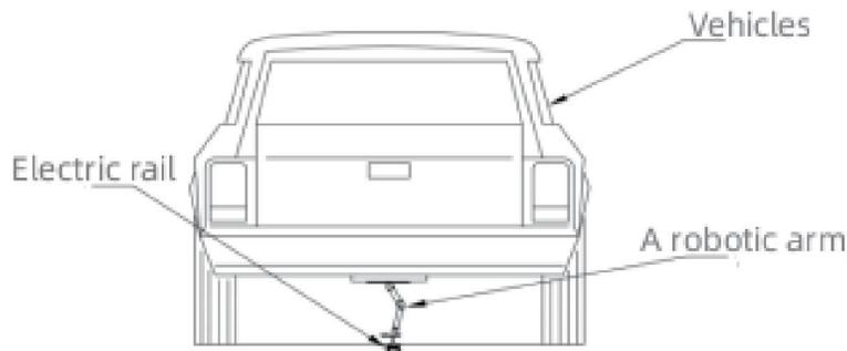
**Figure 2 overall system structure**
