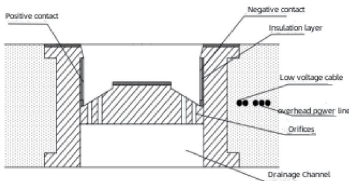
**Figure 3 Schematic diagram of specific structure cross section of charging track**
