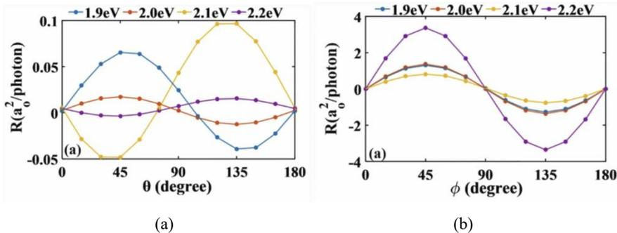
Figure 2. (a) and (b) Photoresponse of linearly polarized light under different polarization angle<sup>[3]</sup>.
