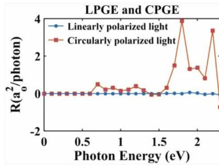
Figure 1. Photoresponse under circularly polarized light and linearly polarized light<sup>[3]</sup>.
