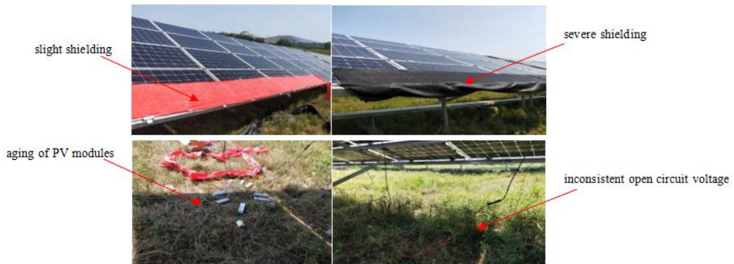
Figure 2. Four test conditions. In order, slight shielding, severe shielding, aging and inconsistent open circuit voltage.
