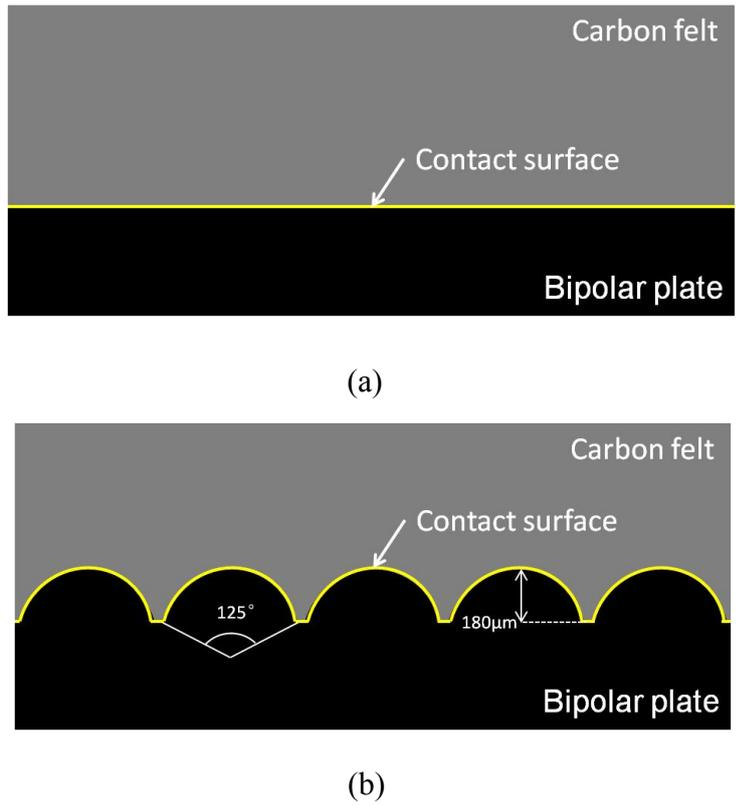
Fig.2. Schematic diagrams of contact areas between the CFE and the BP; (a) smooth contact surface between CFE and the conventional BP, (b) pattern contact surface between CFE and the pattern BP.
