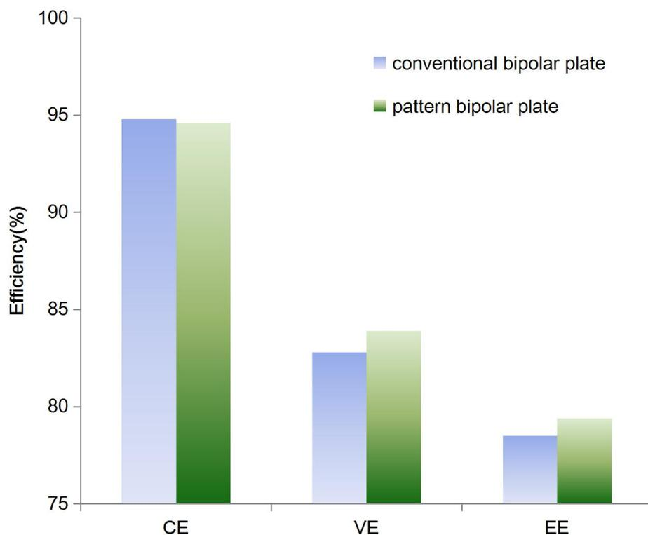
Fig.12. Charge/discharge efficiencies of the pattern bipolar plate and the conventional bipolar plate
