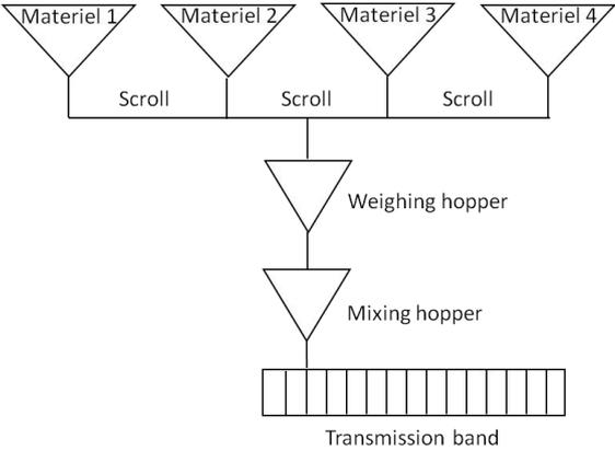
Fig.3. Bipolar plate material mixing system
