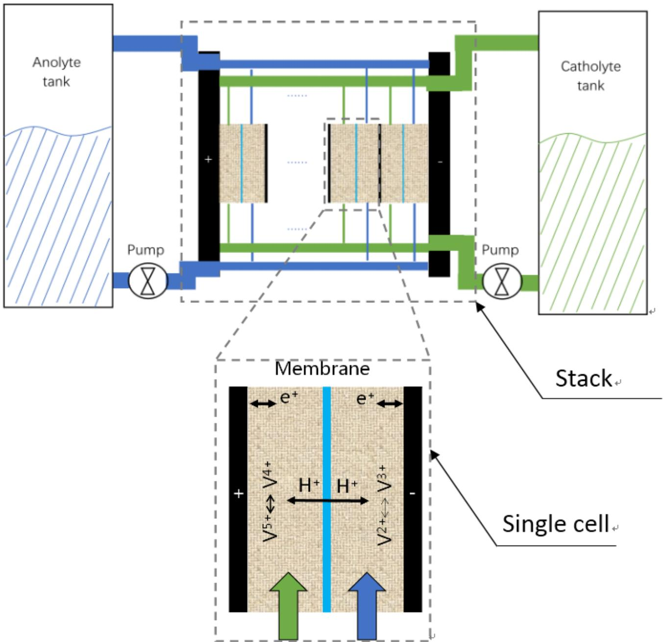
Fig.1. Schematic drawings of vanadium redox flow battery
