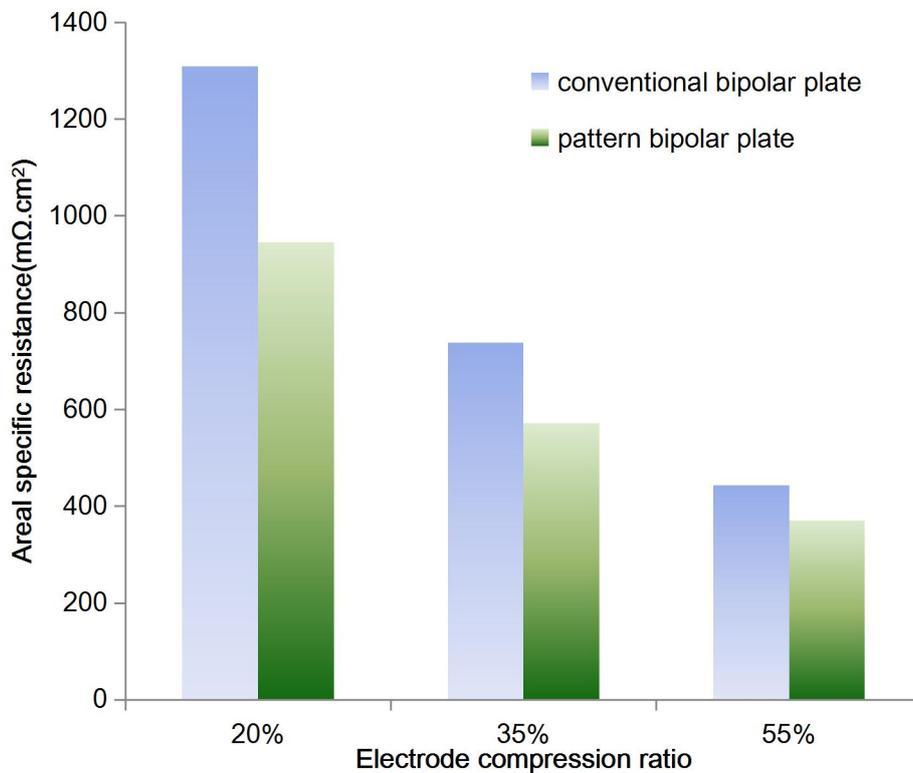
Fig.11. ASRs of conventional/pattern bipolar plate under different electrode compression ratio
