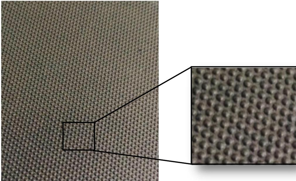
Fig.5. The pattern bipolar plate
