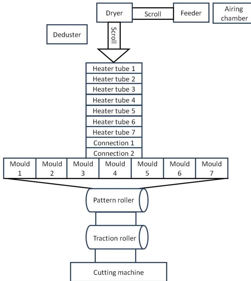
Fig.4. Bipolar plate extrusion system
