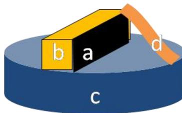
Fig.6. Sample preparation(a: Test sample,b: Conductive support block,c: carrier platform,d: Conductive tape)
