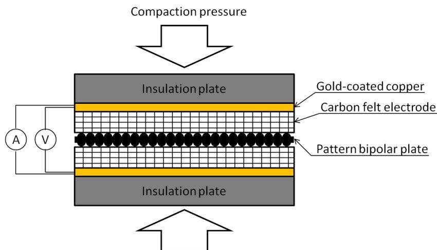
Fig.7. Experimental setup for areal specific resistance measurement
