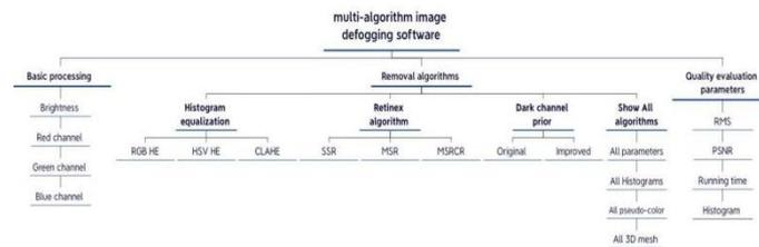
Figure 1 The structure of the multi-algorithm defogging software
