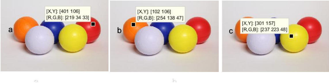
Fig. 3 RGB Values of a) Red Ball, b) Orange Ball and c) Yellow Ball
