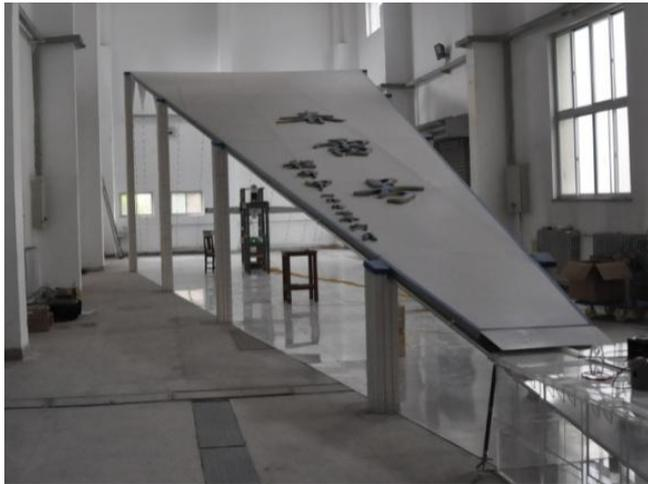
**Fig.11 Bounded wave simulator**
