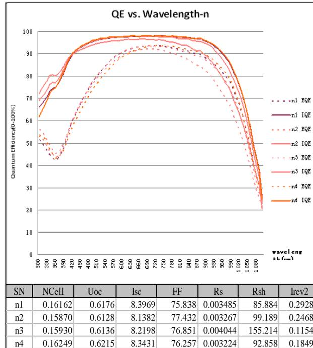
Figure 5. QE test results of cells.
